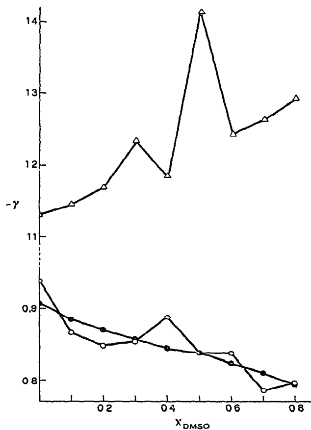
Fig. 1. Variation of the -\gamma values for p -chloro- (○), p -nitro- (●), and p -hydroxybenzoic acid (Δ) as a function of the mole fraction of DMSO at 25°C.
